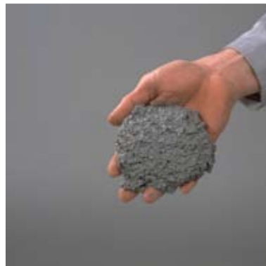
The compound is OK. Ready to install.
