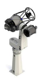
1.2 Automated Telescope Set (ATSold) located at SidingSpring Observatory (Eastern Australia) managed by iTelescope which is a set of two CELESTRON astrograph-based sensors installed on a single PlaneWave L-600 mount with direct drive, cameras, manufacturer's software (Sybilla Technology) and associated cabling and necessary hardware and accessories.
