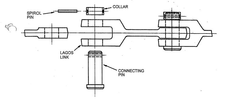
If the fitting of the pins is too difficult an operation to perform inside the casing of the machine it may prove more convenient to suport the links being connected clear of the casing on a bar resting across the side panels. (See diagram below).
