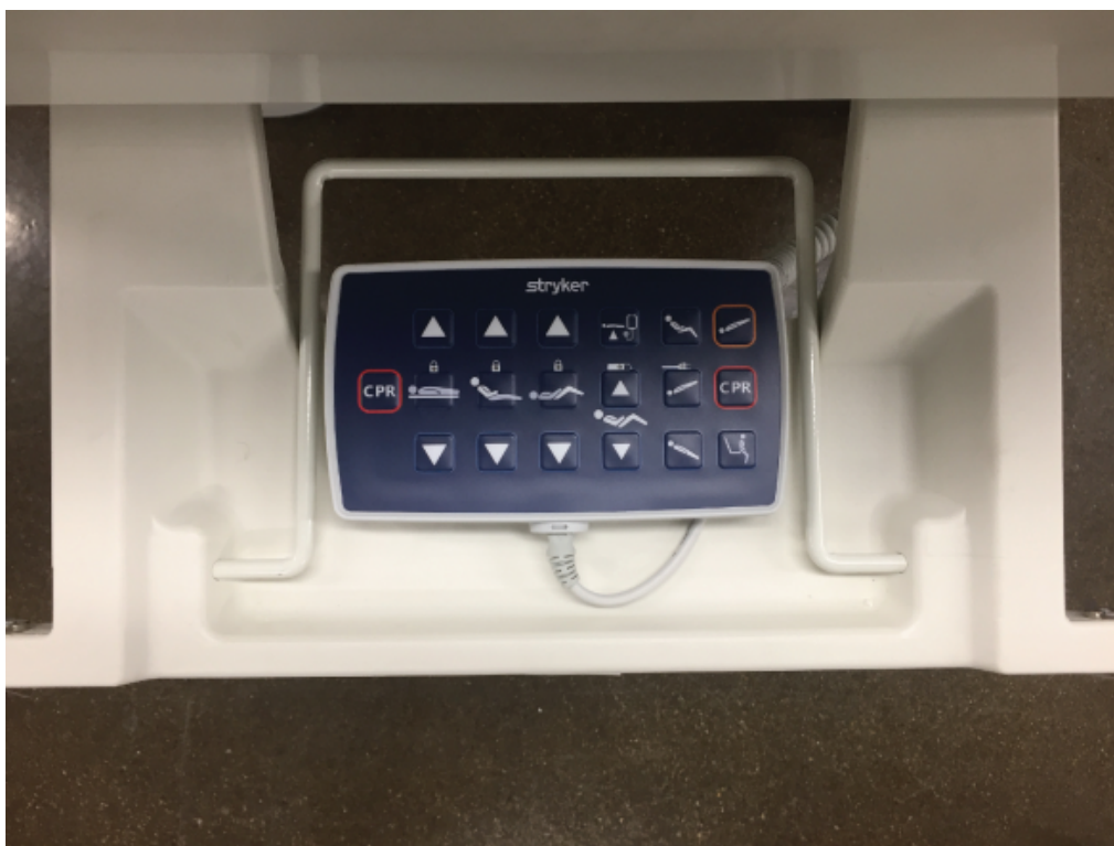
Figure 1-21: Storing the nurse control pendant
