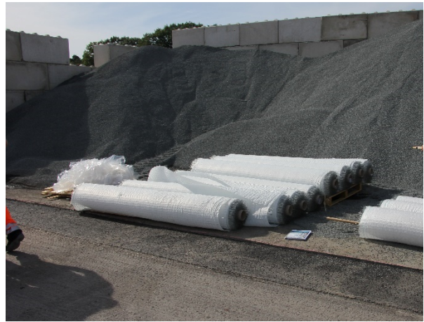
Figure 2: Rolled up / rolls of Fortifix® 1-C (w = 2.66 m)
