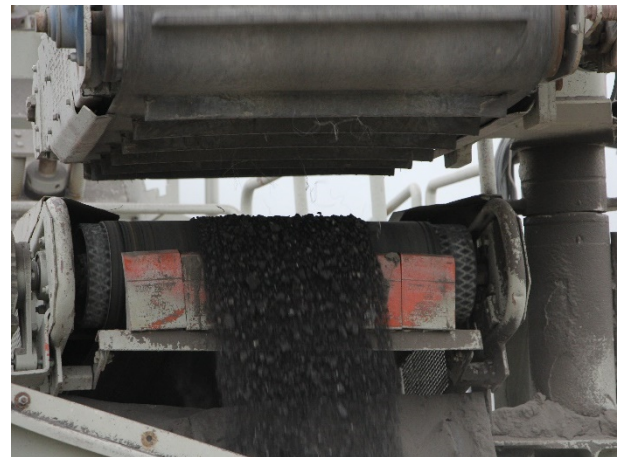
Figure 32: Milled material during reconditioning
