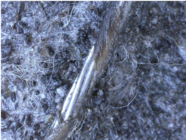
Figure 23: Wire with PET fixation, 20x magnification (on-site)
