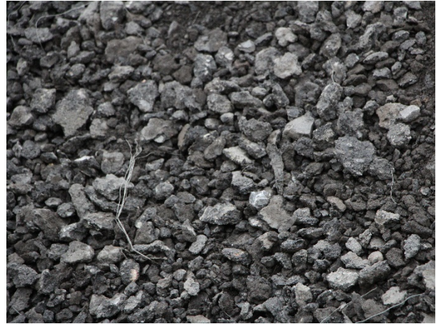
Figure 34: Milled material after reconditioning with larger residual steel cord residues
