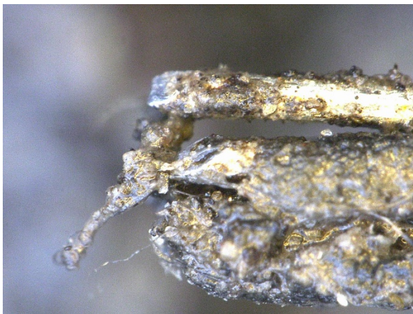
Figure 27: Brittle fracture at the predetermined breaking point, 150x magnification (on-site)
