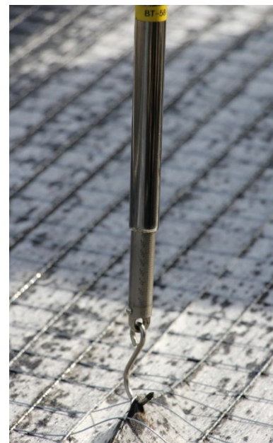
Figure 9: In-situ adhesive bond testing
