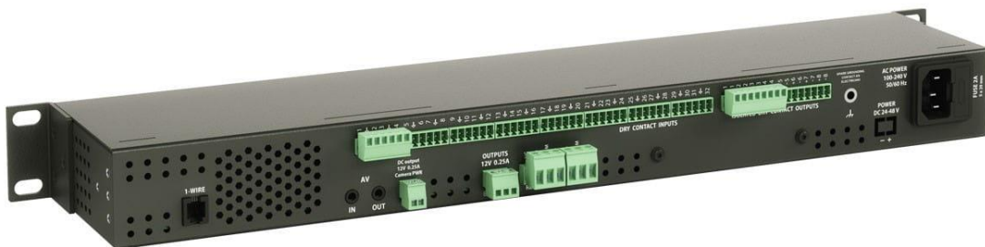
“VT900 / BTS monitoring unit” + “VTX40 / Dry contact board” (all terminals included)
